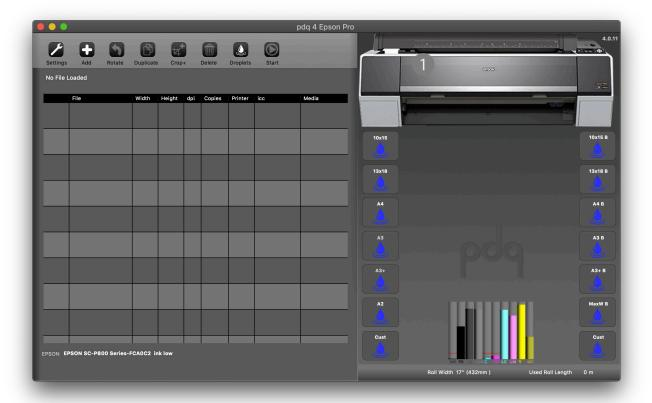
The ink and maintenance cartridge status is also always shown, so you never run out unexpected. When a cartridge drops below 10%, a red line will appear indicating you should prepare to replace that cartridge soon.
